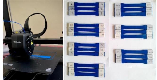
Figure 4: 3D printed tensile specimen
