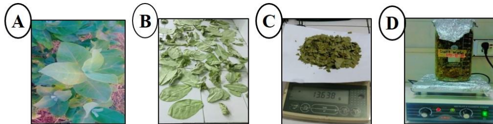
Figure 1. Preparation of leaves extract (A): C. gigantea Plant (B): Dry leaves of C. gigantea (C): Weight the dry leaves (D): Boiled crushed dry leaves on hot plate
