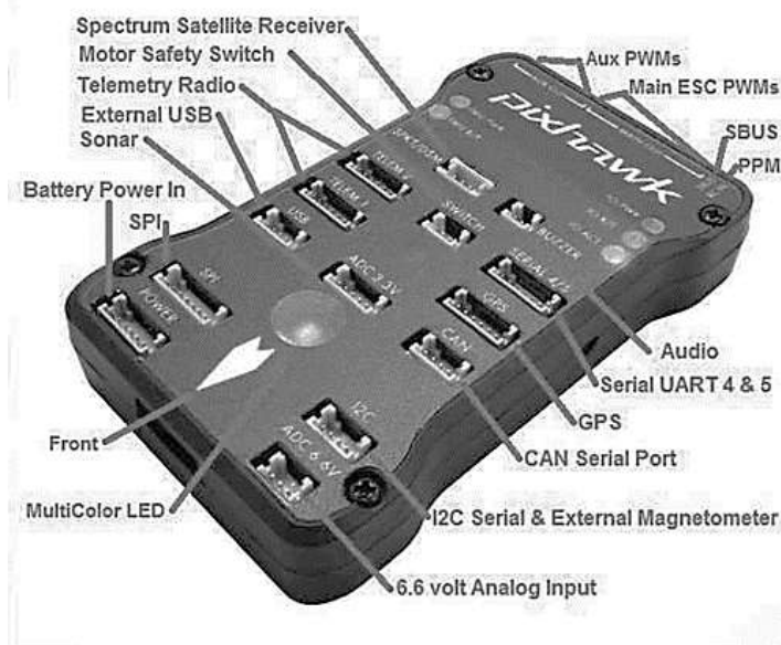
Fig. 2. Pixhawk connection ports [11]
