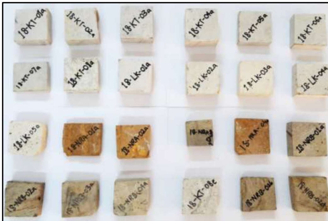
Figure 3. Photographs of representative sedimentary rocks collected from Lower Indus Basin Sindh, Pakistan. Among them KT shows kirthar limestone, LK shows laki limestone, NRA shows nari sandstone and NRB shows nari siltstone
