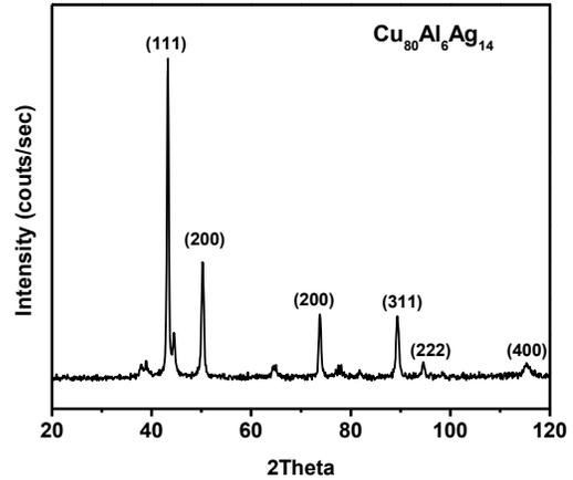
Fig.5. X-ray diffraction pattern of Cu<sub>80</sub>Al<sub>6</sub>Ag<sub>14</sub>
