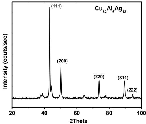
Fig.3. X-ray diffraction pattern of Cu<sub>82</sub>Al<sub>6</sub>Ag<sub>12</sub>
