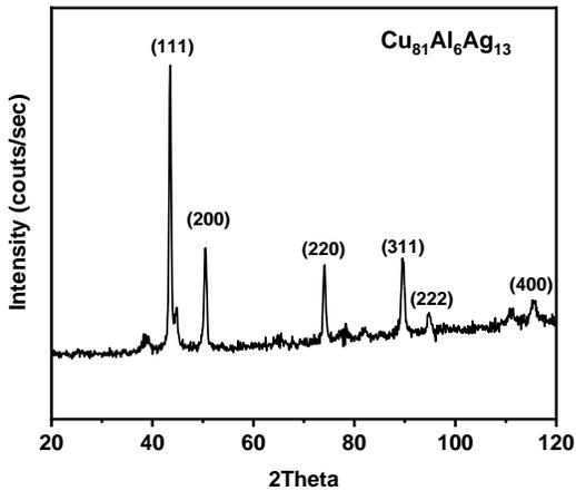
Fig.4. X-ray diffraction pattern of Cu<sub>81</sub>Al<sub>6</sub>Ag<sub>13</sub>
