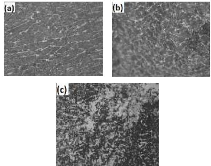
Fig.2. Microstructure of (a)  $\text{Cu}_{82}\text{Al}_6\text{Ag}_{12}$  (b)  $\text{Cu}_{81}\text{Al}_6\text{Ag}_{13}$  and (c)  $\text{Cu}_{80}\text{Al}_6\text{Ag}_{14}$
