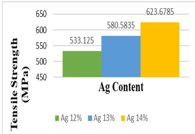
Fig.6. Comparison of Tensile strength in MPa
