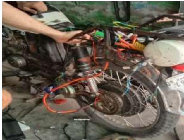
Fig.6 Motor mount built and installed
