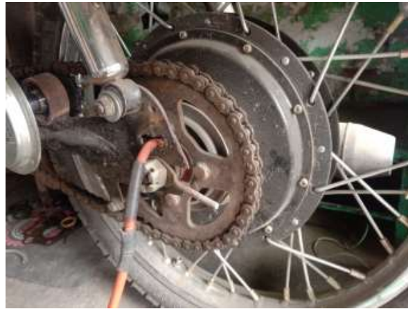
Fig.7 BLDC Motor connection with gear system
