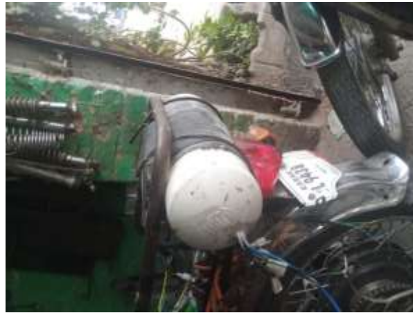
Fig.5 Battery Connection with BLDC Motor
