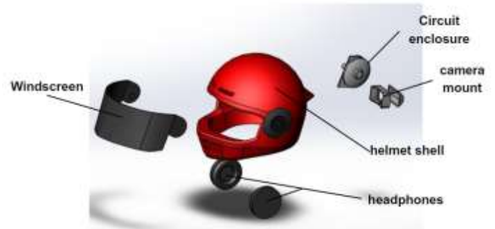
Fig. 1. Conceptual Exploded view of Smart helmet
