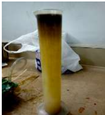
Figure 12 Quantity of Produced Residue oil from the designed model after injection of Alkyl-Benzene-Sulphonate as EOR Fluid
