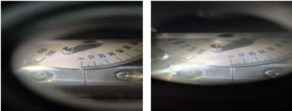
Figure 6 Viscosity calculation of Fluid at 600 and 300 RMP Respectively
