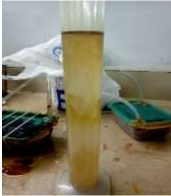
Figure 10 Quantity of Produced Residue oil from the designed model after injection of Saline Water EOR Fluid
