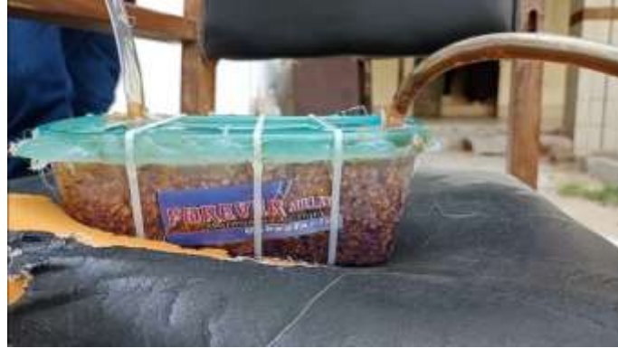
Figure 16 Performing an experiment and injection of LPG as EOR Fluid
