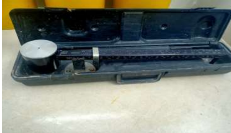
Figure 1 Equipment used to measure the mud Density.
