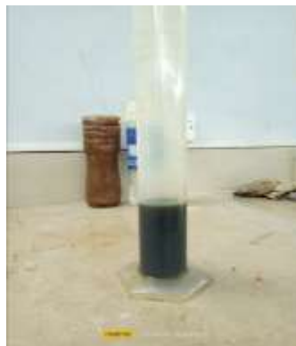
Figure 17 Quantity of Produced Residue oil from the designed model after injection of LPG as EOR Fluid
