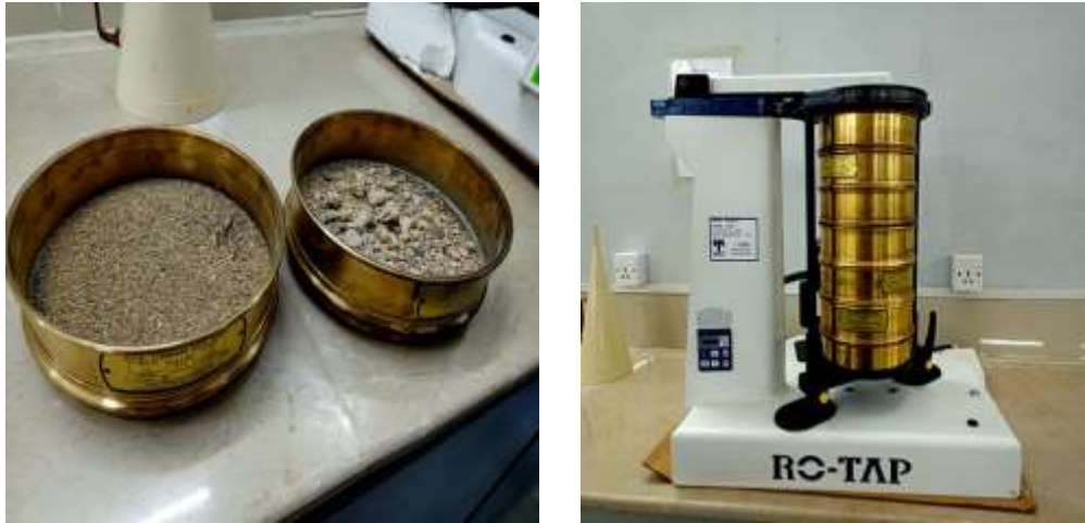
Figure 2 Measurement of Grain Size using Sieve shaker
