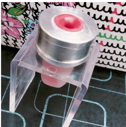
Fig 2: Liquid formulation in a lipstick mold
