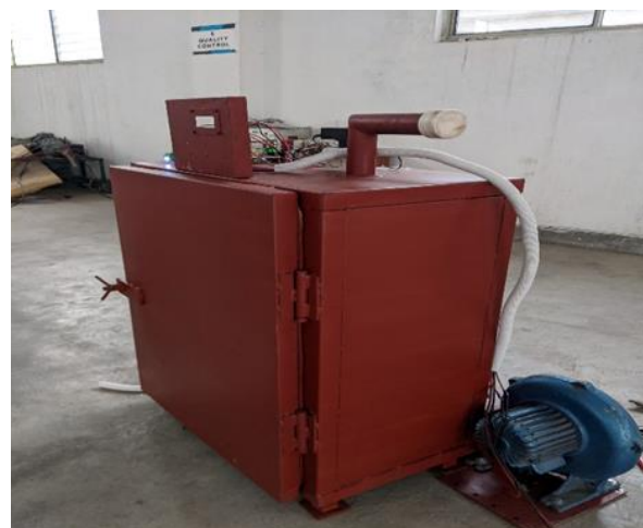
Figure 3: Fabricated Prototype of Petal Drying System
