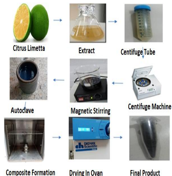
Figure 2.1 Steps for synthesis of nanocomposites
