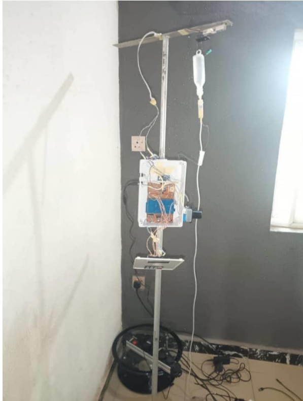
Figure 12: IoT Based Intravenous Fluid Monitor, Air bubble Detector, Blood back flow Detector, Drop rate Regulator, and Alert System
