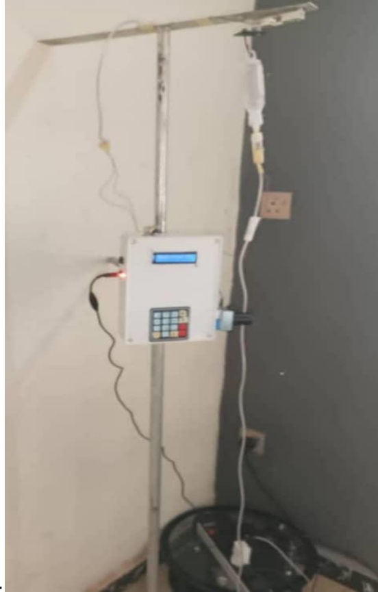
IoT Based Intravenous Fluid Monitor, Air bubble Detector, Blood back flow Detector, Drop rate Regulator, and Alert System
