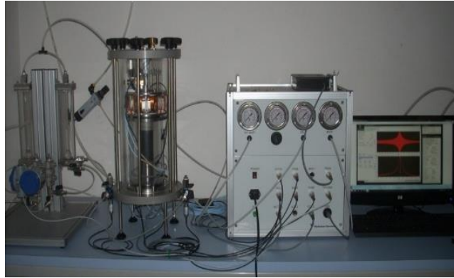
Figure 5. Combine cyclic torsional shear equipment with resonant column
