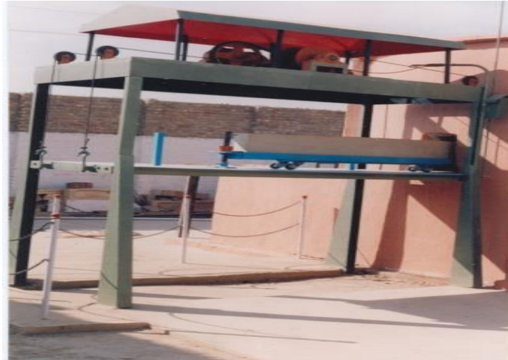
Figure 6. A platform lift placed next to the kiln to safely raise clay beams.
