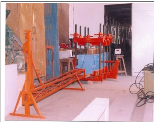
Figure 4. Puller system to remove steel shafts from clay beams after casting.
