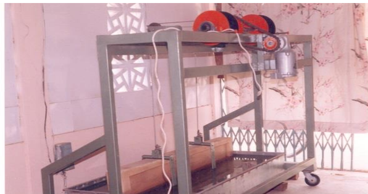
Figure 7. Mobile lift for safe movement of baked clay beams.
