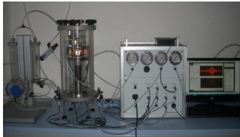
Figure 2. Combine cyclic torsional shear equipment with resonant column
