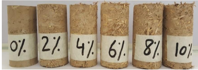
Figure 4. Different wheat straw content % mixed with clayey soil
