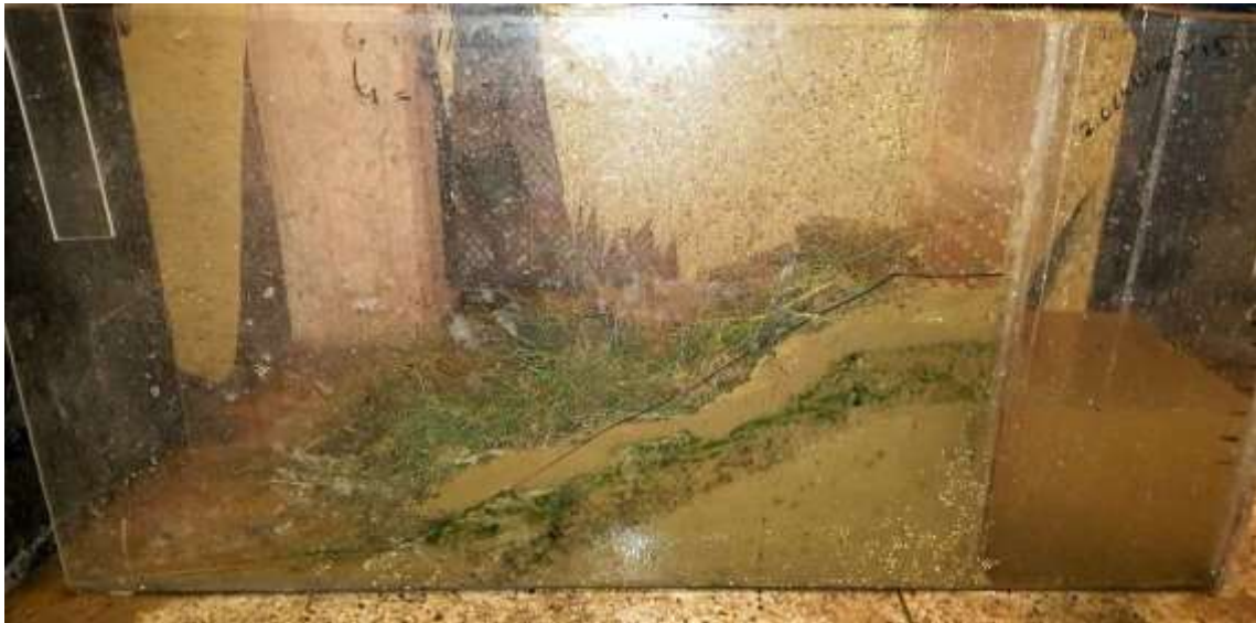
Figure 4. 4: Slope after failure with vegetation cover
