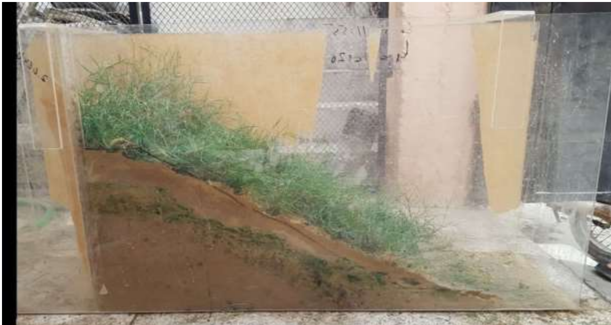
Figure 3. 4 Slope with Vegetation Cover
