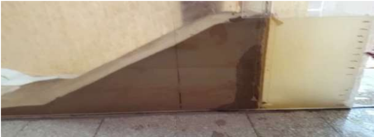
Figure 4. 1: Slope before Failure
