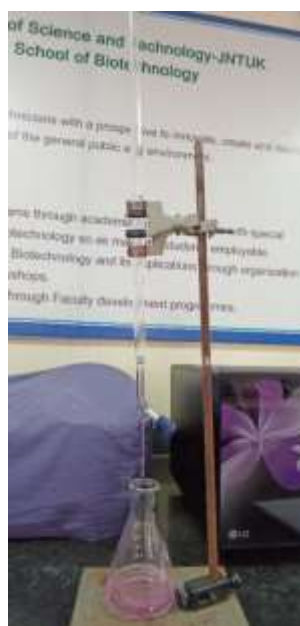
Figure 8: Titration of Biodiesel oil sample for Acid and FFA value
