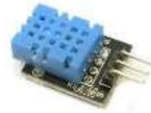
Fig. 13: Temperature &amp; Humidity sensor
