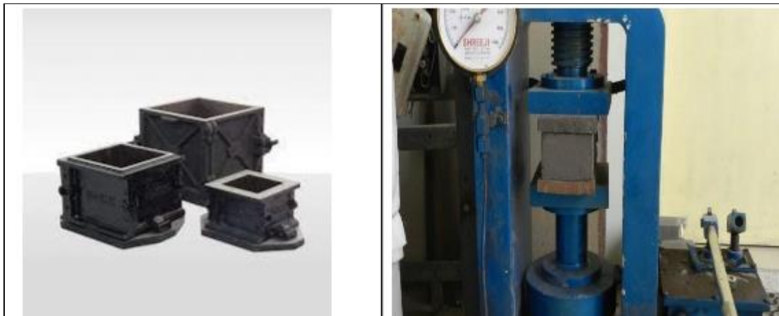
Fig 1 Apparatus for Compressive Strength Test
