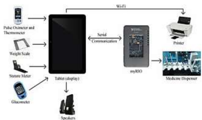
FIGURE 1. Block diagram of myRIO Doc-Dispenser
